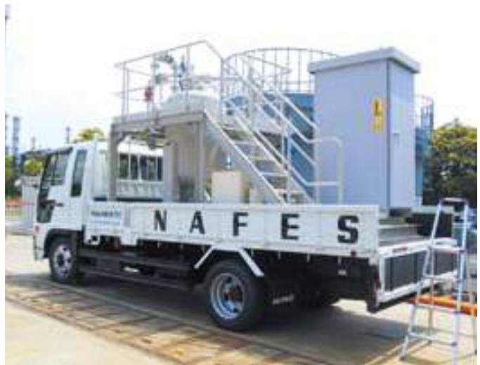
Movable tank-type ferrous ion injection system (movable tank-type "NAFES")
